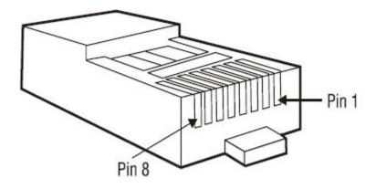
Figure A.1: RJ-45 Pin Assignments
