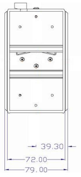
Figure 2.2-3 Rear View of EKI-7559MI/SI
