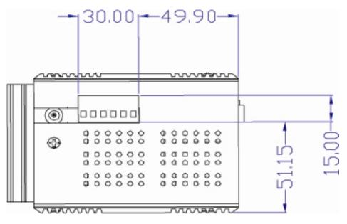
Figure 2.2-4 Top View of EKI-7559MI/SI
