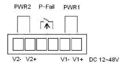
Figure 2.5-1 Pinouts of the Power Connector
